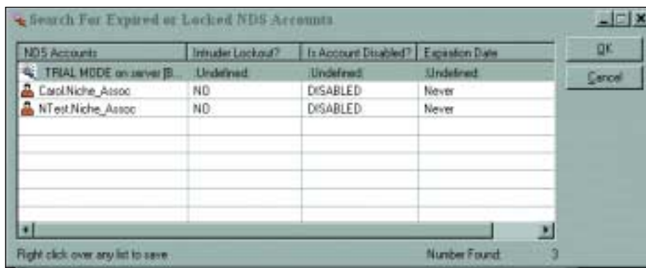
Figure 3. Designer includes a ListView screen control, which supports one Listing service and one or more Display services. This screen control displays information from these services as a report.
