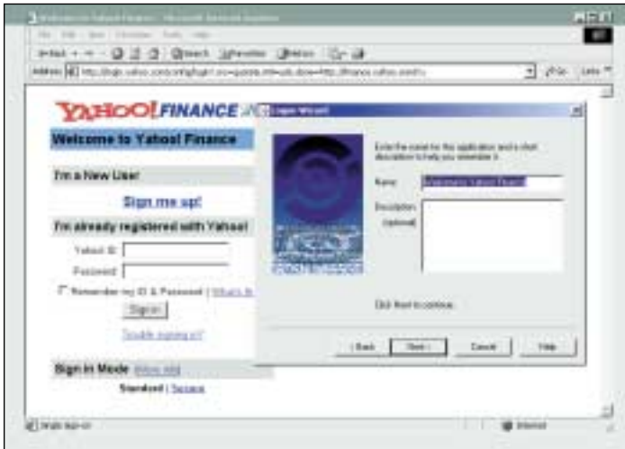
Figure 1. The v-GO Logon Wizard enables users to easily configure Novell Single Sign-on to automatically log in to resources, such as a web site, that require a username and password.
