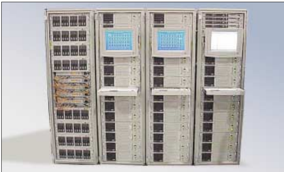
Figure 3. At BrainShare 2000, Novell engineers demonstrated two 32-node clusters. This cluster featured four Compaq ProLiant 1850R servers and 28 Compaq ProLiant DL380 servers connected via Fibre Channel to eight Compaq RAID Array (RA) 4100s. (In case you are counting and curious, the racks also held five additional Compaq ProLiant 1850R servers, as well as four beta Compaq ProLiant DL360s, but these were used for other purposes.)
