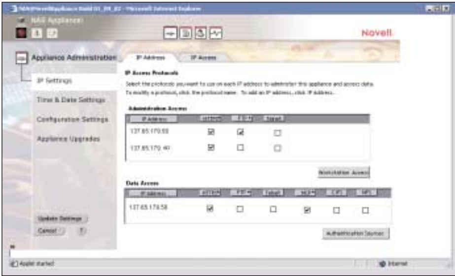
Figure 4. The Novell Network Storage Appliance includes a GUI management tool. This figure shows a sneak peek at a beta version of the IP Access configuration page, through which you select the protocols that you want to use to manage the appliance and access data.
