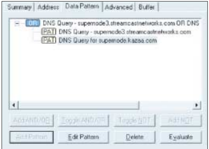
Figure 4. To catch Morpheus traffic based on the application-level calls, you build a filter that looks for the Morpheus client's DNS queries.
