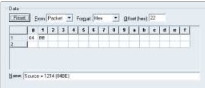
Figure 2. This filter is for Morpheus traffic. The hexadecimal value 0x04BE is equivalent to the decimal value 1214.
