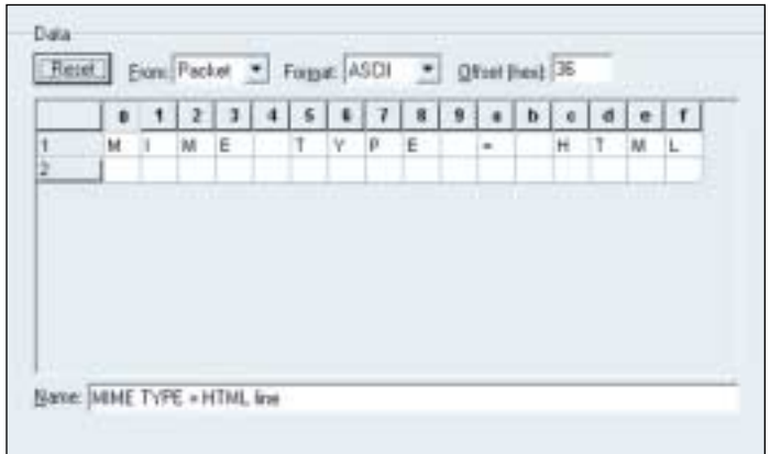
Figure 9. The only command that can be identified in the iMesh traffic is a reference to the “mime type.”
