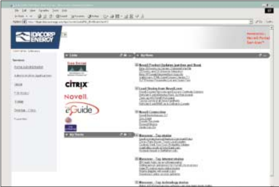
Figure 1. To provide secure remote access to network information and services, IDACORP Energy uses Novell iChain and Novell Portal Services. Users first authenticate to iChain. iChain then displays the company's Novell Portal Services portal, through which these users can access the information and services that they are authorized to receive.
