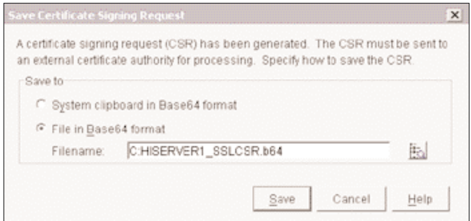
Figure 1. When you save the CSR, you should save it in Base 64 format.
