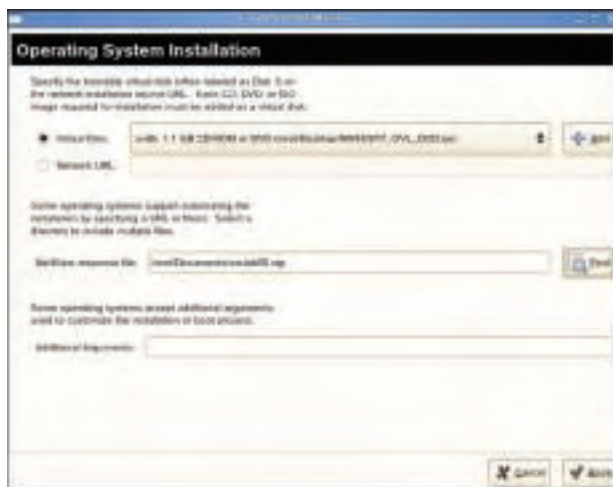
Figure 4 Using a response file during the installation of a NetWare virtual machine can be useful when you need to create multiple NetWare virtual machines.
