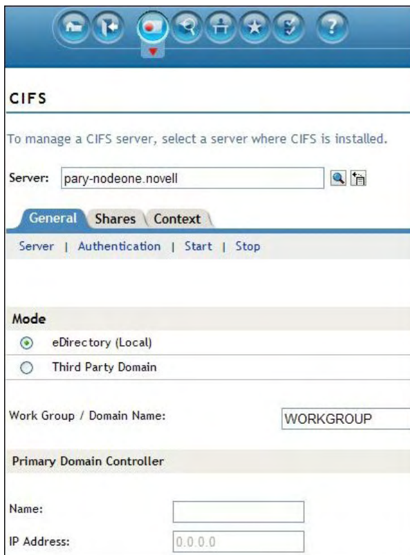
Figure 2: The CIFS support in OES 2 support pack 1 enables users to access a Linux server from a Windows client with the same look and feel as if they were accessing a NetWare server.
