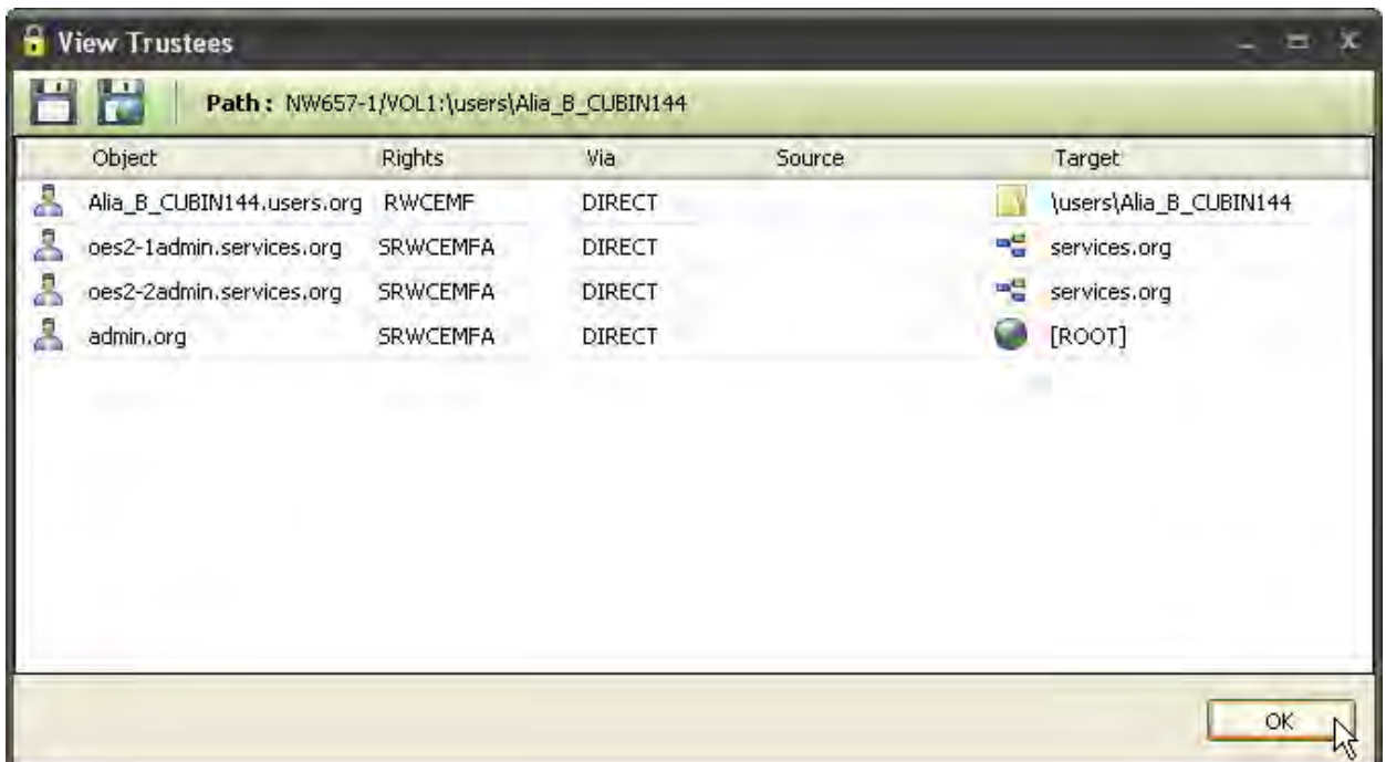
Figure 2: Path Analysis can quickly and easily show who has access rights to a particular directory.
