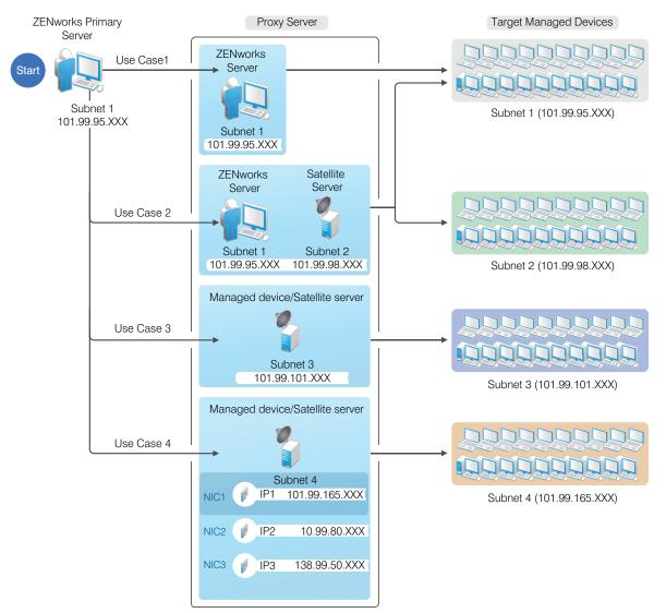
This diagram shows Subnet 1, Subnet 2, Subnet 3, and Subnet 4 respectively. All devices that are located in these four subnets are managed by a ZENworks Primary server located in Subnet 1.
