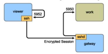
Windows Console to Linux managed device with tunneling
