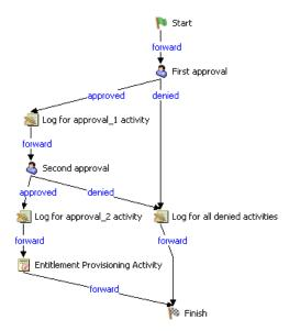
Figure 4-3 Parallel Workflow with Two Approvals
