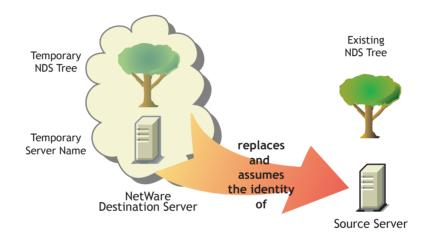
Before you can migrate your data, you must first install a destination NetWare server in a temporary eDirectory tree. A temporary eDirectory tree is simply a tree that contains one server with a basic installation of NetWare and no additional products installed (other than SMS<sup>™</sup> or any other default products).
