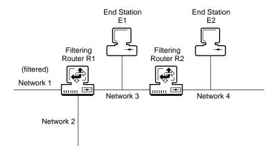
The route to Network 1 is filtered out in Router R1's advertisement to Network 3. If End Station E2 sends a packet to Network 1, Router R2 drops that packet because it does not have a route. If End Station E1 sends a packet to Network 1, Router R1 forwards it because it does have a route. End Station E1 can send a packet to Network 1 only if it has a route to that network. End station E2 can see only Networks 2, 3, and 4. End station E1 can see both Networks 1 and 2.
