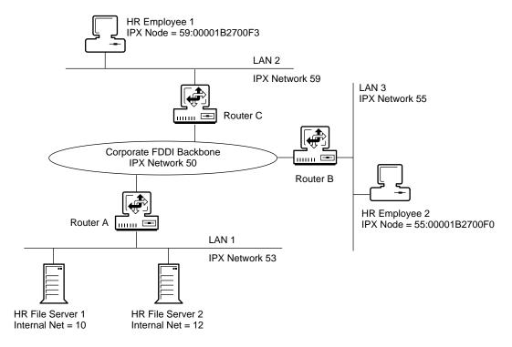
Routers B and C do not require filters because users can access all corporate servers (except for the HR server). Packet forwarding filters are installed on Router A to block packets from the FDDI interface to the HR servers, except when the packets are from the nodes 59:00001B2700F3 and 55:00001B2700F0.
