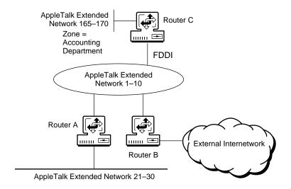
Extended network 165-170 can be hidden from the rest of the organization if an outgoing route filter is configured on Router C.
