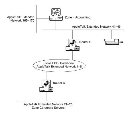
All networks within the Accounting department are in Zone Accounting. A device hiding filter on Router C stops access from specific areas to the LaserWriter\* printers within the Accounting zone.
