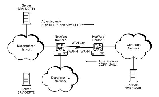
To minimize the load on the WAN link, an IPX SAP filter is configured on Router 1 and Router 2. This filter cuts down the periodic service information updates across the WAN link by advertising only a few selected servers. The clients across the WAN link can access the servers on the other network by first attaching to these selected servers.
