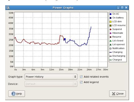
Figure 1-20 Power History Going From Battery Power to AC
