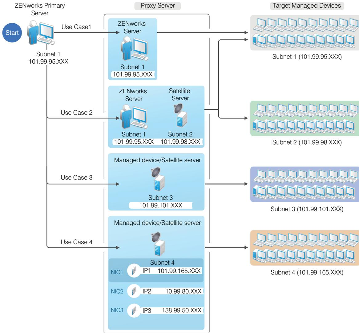
This diagram shows Subnet 1, Subnet 2, Subnet 3, and Subnet 4 respectively. All devices that are located in these four subnets are managed by a ZENworks Primary server located in Subnet 1.
