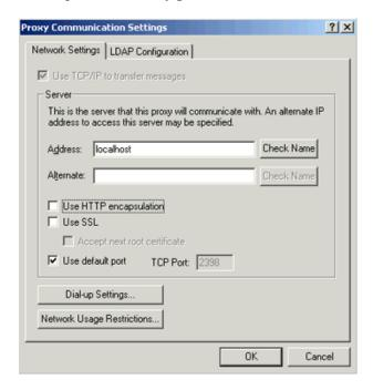
Alternate addresses can be defined for the server when the server is on a network that defines one set of IP addresses for internal traffic and another set of IP addresses for traffic from outside of the firewall, for instance when you are using Network Address Translation (NAT).
