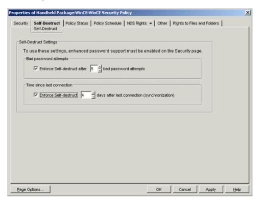
The *Self-Destruct* page lets you configure self-destruct settings for Windows CE devices so that data is not accessible from handheld devices that are lost or stolen. When the self-destruct feature is activated, the data on the device is made unusable and the device must be manually reset, which restores the device to its out-of-the-box state.
