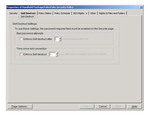
The *Self-destruct* page lets you configure self-destruct settings for Palm OS devices so that data is not accessible from handheld devices that are lost or stolen. When the self-destruct feature is activated, the data on the device is made unusable and the device must be manually reset, which restores the device to its out-of-the-box state.
