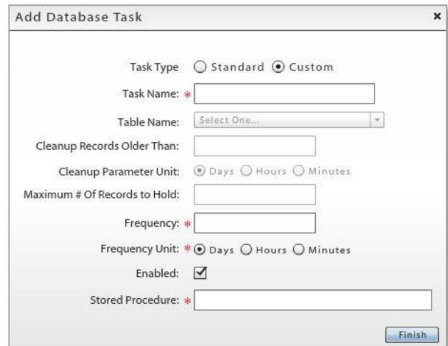
The screenshot shows the 'Add Database Task' dialog box with the 'Custom' radio button selected. The fields are: Task Name (text input), Table Name (dropdown menu), Cleanup Records Older Than (text input), Cleanup Parameter Unit (radio buttons for Days, Hours, Minutes), Maximum # Of Records to Hold (text input), Frequency (text input), Frequency Unit (radio buttons for Days, Hours, Minutes), Enabled (checked checkbox), and Stored Procedure (text input). A 'Finish' button is at the bottom right.
