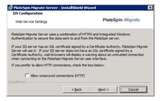
If you require unsecured connections (HTTP), select the *Allow unsecured connections* (HTTP) option; if you require secured connections (HTTPS), leave the option deselected (default).
