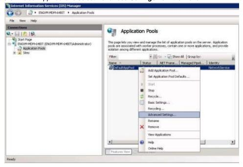
5. Under the *Process Model* section, adjust the *Maximum Worker Processes* to a value greater than 1, (see the recommendations listed earlier in this section). The value should remain at 1 for a non-Web garden setup or on single core machines.
