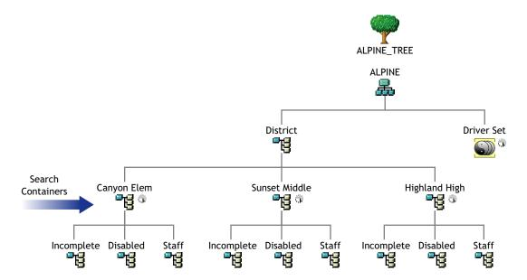
In this example there are three Zones, one per school. Identity Manager and the DirXML Driver for SIF are installed on a server that holds replicas of the partitions from each school. One driver is configured to connect to all three Zones.
