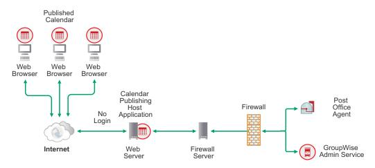
The firewall must allow inbound IP packets to be sent from the web server to the POA's internal or external IP address and the calendar publishing port for the POA (for example, 172.16.5.18:7171). If you are using an external IP address, all POAs that support calendar publishing must be configured to use the same external IP address. For more information about external POA IP addresses, see "Securing Client Access through an External Proxy Server" in the *GroupWise 2014 R2 Administration Guide*.
