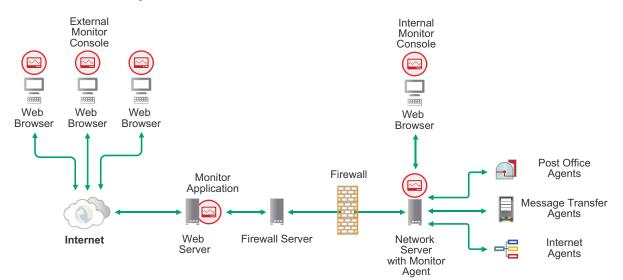
The firewall must allow inbound IP packets to be sent from the web server to the IP address and port number of the Monitor Agent (for example, 172.16.5.18:8200).
