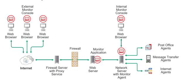
If desired, the Monitor Agent can also be installed to the web server rather than to a separate server, as described in "One Monitor Server versus Two" on page 132.
