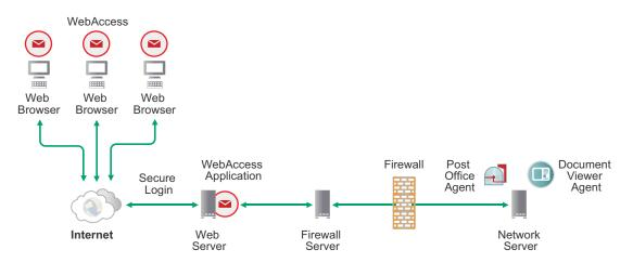
The firewall must allow inbound IP packets to be sent from the web server to the IP address and port of the POA (for example, 172.16.5.18:1677).
