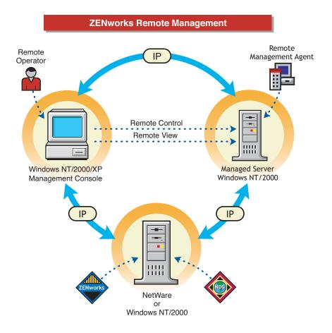
To remotely manage a server, the ZENworks 6.5 Remote Management Agent component must be installed on that server. For more information, see "Policy-Enabled Server Management Installation" in the Novell ZENworks 6.5 Server Management Installation Guide.
