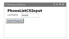
When the user submits the form, the service executes. When the service has finished processing, the pageflow displays an output form that shows the data returned by the service.
