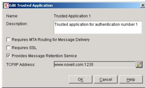
When ConsoleOne reads a trusted application record that has the Provides Message Retention Service setting turned on, it adds a Retention tab to the GroupWise Client Environment Options (Tools > GroupWise Utilities > Client Options > Environment).
