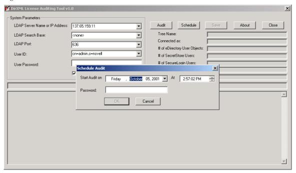
Specify a start date and time. The password entered in the password field will become the key to unlock the DLAT's UI. After filling in the dialog box, click OK to schedule the audit event and lock the UI to prevent tampering with the audit parameters or results.
