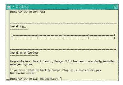
eDirectory temporarily shuts down when installing the Metadirectory Engine and schema files. By default, all available drivers are installed so you won't need to run the installation program later if you want another driver. The driver files are not used until a driver is configured through iManager or through Designer and then deployed.
