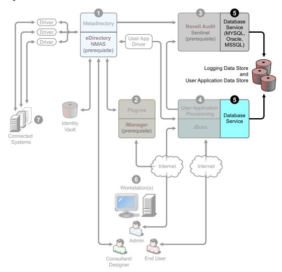
The secure logging service does not include a specific database. However, you can use the MySQL database that comes with the User Application and provisioning. The User Application comes with the JBoss Application Server Version 4.2.0, and the User Application requires JRE\* 1.5.0\_10. To install this service, see Section 5.3, "Installation and Configuration Steps," on page 107.
