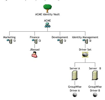
In this example, the Identity Manager administrator has two Identity Vault servers, Server A and Server B, shown in Figure 2-6 on page 60. Neither server contains a copy of all the users. Each server contains two of the three partitions, so the scope of what the servers hold is overlapping.
