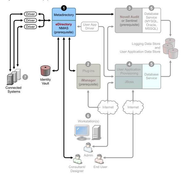
When data from one system changes, the Metadirectory engine included in Identity Manager detects and propagates these changes to other connected systems based on the business rules you define. This solution enables you to enforce authoritative data sources for any particular piece of data (for example, an HR application owns a user's ID, while a messaging system might own a user's e-mail account information).
