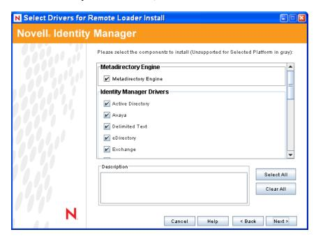
The Select Drivers for Engine Install page shows you which drivers can be installed on a corresponding platform. By default, all available drivers are selected.
