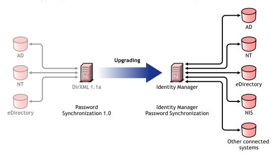
Identity Manager Password Synchronization offers many features, including bidirectional password synchronization, additional platforms, and e-mail notification when password synchronization fails.
