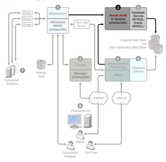
Repository for logging events (Identity Manager software is not installed on this server, but having a secure logging service is mandatory). This is a central service that is used by Identity Manager and the user application and workflow system services and is downloaded separately from the Novell Download Web site (http://download.novell.com).
