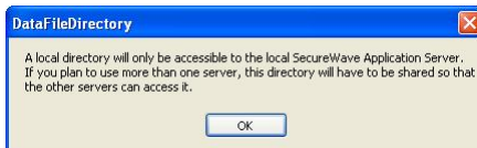
Figure 26: SecureWave Application Server installation: warning message when setting the log files folder to a local drive
