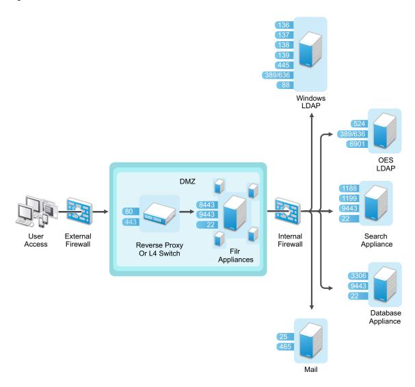
Only traffic destined to the DMZ is allowed through the front-end firewall, and only traffic from the DMZ to the internal network is allowed through the back-end firewall.
