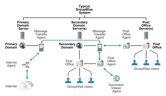
Messages are moved from user to user through your GroupWise system by the GroupWise agents. As illustrated above, each domain must have a Message Transfer Agent (MTA). The MTA transfers messages between domains and between post offices in the same domain. Each post office must have a Post Office Agent (POA). The POA delivers messages to users' mailboxes and performs a variety of post office and mailbox maintenance activities.
