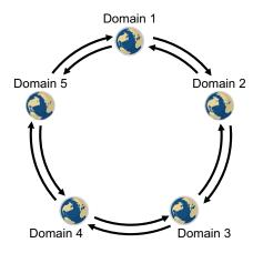
An advantage of the two-way ring configuration is that it has no single point of failure. A disadvantage is that, depending on the size of the system, a message might go through several domains before arriving at its destination. A two-way ring works well in a system with five domains or less because transferring a message never requires more than two hops.
