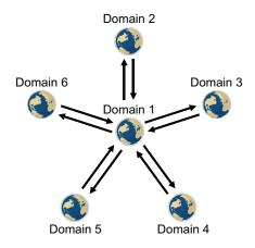
If you have more than ten domains, you might want to designate the central domain as a routing domain. The sole function of a routing domain is to transfer messages between other domains; it has no post offices of its own. See Configuring a Routing Domain.
