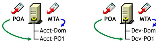
Running the MTA on a remote server allows you to place the heaviest processing load on your highest performing server. In the following diagram, the agent software is installed on a different server from where the domains and post offices reside.
