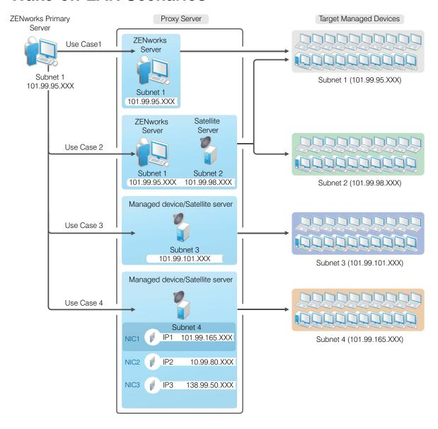
This diagram shows Subnet 1, Subnet 2, Subnet 3, and Subnet 4 respectively. All devices that are located in these four subnets are managed by a ZENworks Primary server located in Subnet 1.
