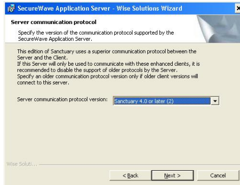
Figure 29: SecureWave Application Server installation: protocol selection dialog
