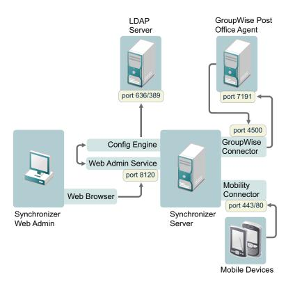
The GroupWise Connector initially communicates with the POA that you specify during Mobility Pack installation on the SOAP port that you specify. As users connect their mobile devices, the GroupWise Connector determines from the initial POA the IP addresses and port numbers of all POAs where mobile device users have their mailboxes. Therefore, the GroupWise Connector can communicate with multiple POAs throughout your GroupWise system.
