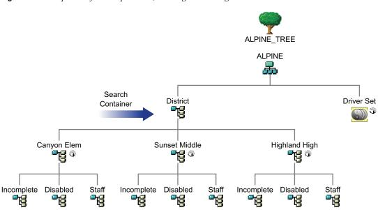
In this example there are three Zones, one per school. Identity Manager and the Identity Manager Driver for SIF are installed on a server that holds replicas of the partitions from each school. One driver is configured to connect to all three Zones.
