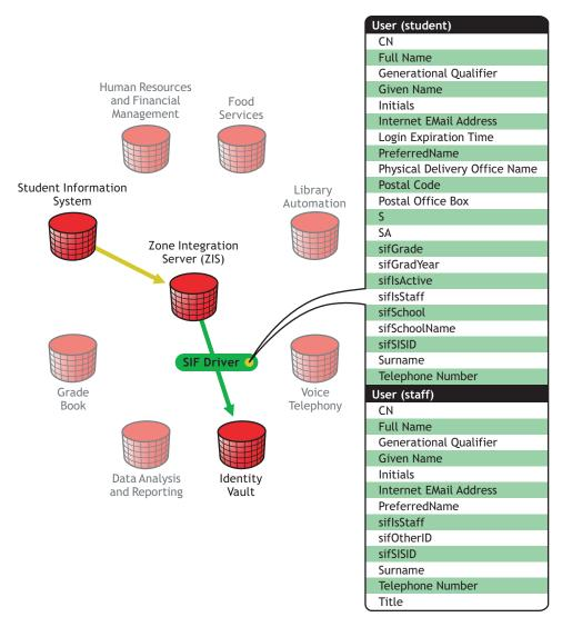
In the driver configuration provided, the Identity Vault receives information from the Student Information System. You can customize the configuration to change how students and staff are provisioned, and cause the Identity Vault to send information to the ZIS.
