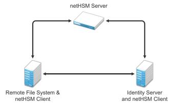
Access Manager allows you to use netHSM to store and manage the signing key pair of the Identity Server. You must use the Administration Console to store and manage the other Access Manager certificates. Access Manager uses the Java Security provider of the netHSM server to interact with the netHSM server.
