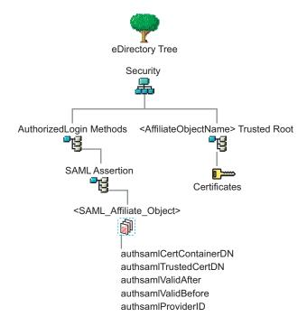
If the schema has been extended correctly, you can find a SAML Assertion object in the Authorized Login Methods container. The SAML\_Assertion object contains an alphanumeric generated name for a SAML affiliate object. This object has four attributes.
