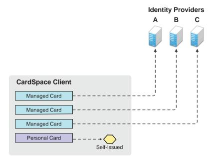
Managed cards come from an identity provider. When the users interact with the Identity Server, they can install a managed card from the Identity Server into the CardSpace client. The managed card provides metadata to CardSpace about how to interact with the Identity Server, which includes the available attributes (claims).
