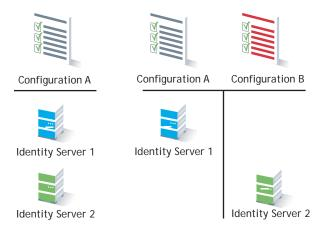
When you assign multiple Identity Servers to the same configuration, you need to install a load balancer that supports either Layer 4 or Layer 7. This device is referred to as an L4 switch in this manual. The L4 switch allows the work load to be balanced among the machines.
