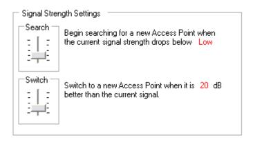
Figure 86: Signal Strength Control
