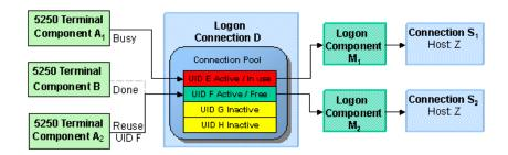
In this diagram, Logon Connection D is associated with four connections based on four UIDs (user IDs or credentials: A-thru-F). One is in use; another (UID 'F') is alive but not being used; and two are inactive but available (i.e., valid UIDs have been assigned, so these two connections can be made live at any time).
