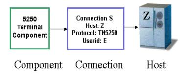
The TN5250 connection resource is designed to make an individual connection to the host on an as-needed basis. The connection is made just-in-time and discarded as soon as the client is done. It is not reused in any way. This is the type of connection resource we created in Chapter 2 of this Guide.
