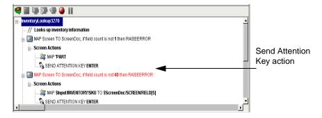
Double-clicking the Send Attention Key action in the Action Model displays a dialog box that allows you to edit the key. Select from the dropdown list box the Value Key. Click on the checkbox to override the cursor position. Edit the row and column if needed or click on the expression builder icon to add a calculation.
