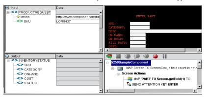
**5** Drag the SKU data from the Input DOM to the SKU field in the 5250 ENTER PART screen. The action is recorded in the Action Model pane and appears in the status bar.
