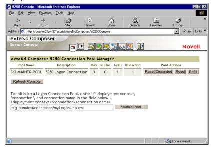
To initialize a Logon Connection Pool, enter its deployment context, the word "connection", and the actual connection name in the text field near the bottom of the screen. (See illustration above.) Then click the **Initialize Pool** button.
