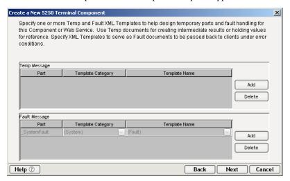
**9** If desired, specify a template to be used as a scratchpad under the "Temp Message" pane of the dialog window. This can be useful if you need a place to hold values that will only be used temporarily during the execution of your component or are for reference only. Specify the templates as indicated in Step 6 above.
