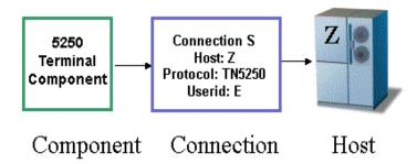
The TN5250 connection resource is designed to make an individual connection to the host on an asneeded basis. The connection is made just-in-time and discarded as soon as the client is done. It is not reused in any way. This is the type of connection resource we created in Chapter 2 of this Guide.
