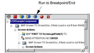
5 Click the **Run to Breakpoint/End** button. The Action Model executes all of the actions from the beginning to the breakpoint you set in step 3 above and appears as shown.
