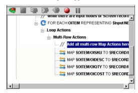
Notice that Map actions within the Multi Row actions block reference fields by their relative position in the row and not their absolute position within the screen. So the target of the first Map action is \$RECORD/FIELD[1]. Using drag and drop to create your Map actions within the context of the Multi Row will create and assign these field indexes for you automatically.
