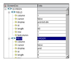
In the sample list of ScreenDoc Fields in the above graphic, the XPath location ScreenDoc.XPath ("SCREEN/FIELD[@cursor= 'true']/@id") would return the number "4" indicating that Field 4 is the current cursor location.
