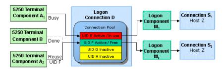
In this diagram, Logon Connection D is associated with four connections based on four UIDs (user IDs or credentials: A-thru-F). One is in use; another (UID 'F') is alive but not being used; and two are inactive but available (i.e., valid UIDs have been assigned, so these two connections can be made live at any time).
