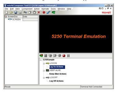
**NOTE:** Recording actions follows a series of steps. The cursor must be positioned over Logon; turn Record on; when you are done, turn Record off. Position the cursor to KeepAlive; turn Record on; when you are done, turn Record off. Position the cursor to Logoff; turn Record on, when you are done, turn Record off.
