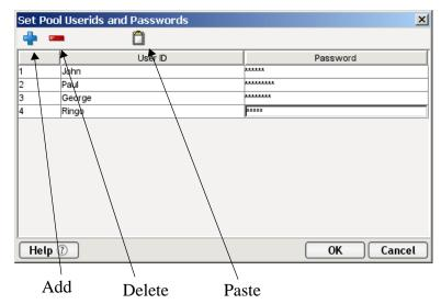
On the Toolbar there are three icons: Add which adds an empty row, Delete, which deletes a highlighted row and Paste which allows you to copy/paste information from a spreadsheet into the table.
