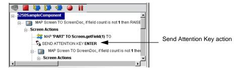
Double-clicking the Send Attention Key action in the Action Model displays a dialog box that allows you to edit the key. Select from the dropdown list box the Value Key. Click on the checkbox to override the cursor position. Edit the row and column if needed or click on the expression builder icon to add a calculation.
