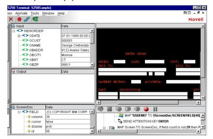
The applicable header data is dragged and dropped from the input DOM to the corresponding field in the 5250 ENTER ORDER screen:
