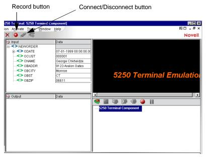
**NOTE:** In addition to the buttons found on the XML Map Component Editor tool bar, the 5250 Component Editor includes a **Record** and **Connect/Disconnect** button as shown above.
