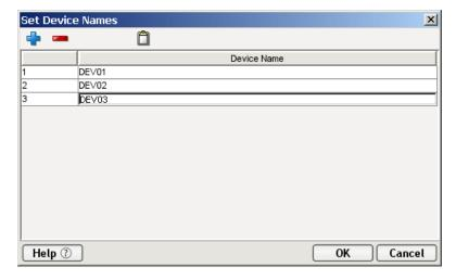
On the Toolbar there are three icons: Add which adds an empty row, Delete, which deletes a highlighted row and Paste which allows you to copy/paste information from a spreadsheet into the table. For more on this, see the following Note.
