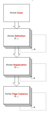
**Portlet class** The Java class that defines the initialization parameters and default behavior of the portlet. Each portlet class in a portlet application must have a definition descriptor to make the portlet available to the portlet container. These descriptors must be created either as an entry in portlet.xml or as a separate portlet fragment deployment descriptor, as described in the section on portlet application deployment descriptors.
