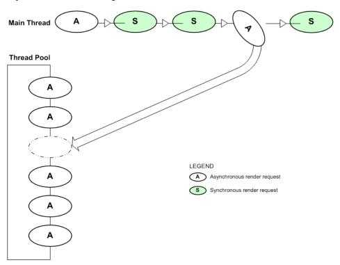
By default, the exteNd Director portal assigns each asynchronous render request to its own thread in the portlet thread pool. When all threads in the pool have been assigned, incoming asynchronous render requests are delegated to the main request thread, as described in "The main request thread" on page 174.
