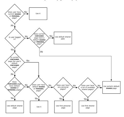
As the flow diagram shows, the Portal Aggregator checks for the following shared or personal pages:
