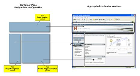
In this example, a portal administrator configures a container page with a Header-Navigation-Content layout and three system portlets:
