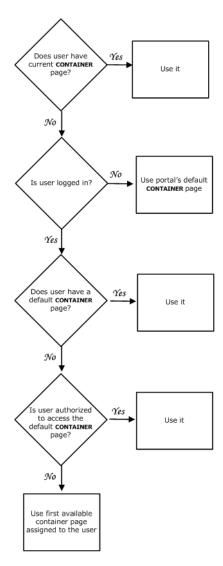
As the flow diagram shows, the Portal Aggregator checks for the following container pages:
