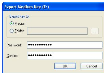
Figure 133: The Export Medium Key dialog to export the encryption key on the device itself
